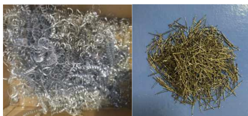
Fig. 1. Fibers used. Aluminum fibers (left); b) Steel fibers (right).
