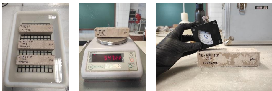
Fig. 1. Test performed: Open porosity and surface hardness. (Source: Own production)
