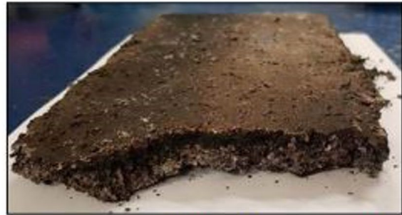
Gypsum panels added with plastic waste during direct fire test (left) and after test (right)
