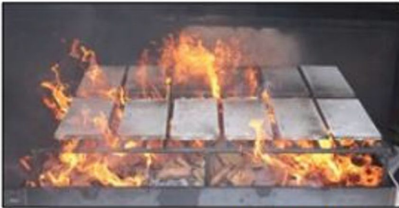
Gypsum panels added with plastic waste during direct fire test (left) and after test (right)
